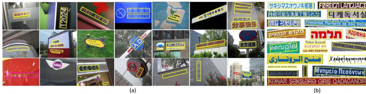
Figure 8. (a) Detected texts in images from the proposed dataset. Yellow rectangles: true positives, pink rectangles: false negatives, red rectangles: false positives. Best viewed in color. (b) Detected texts in various languages in images collected from the internet. Note that the texts are detected in full images. We only show cropped sub images because of space limitation.
