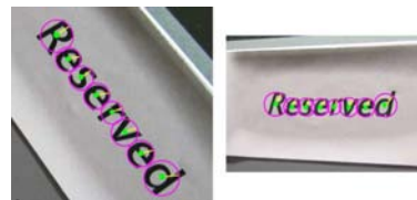
Figure 4. Component characteristics. The green points are the centers of the components. The radii of the pink circles represent their characteristic scales while the yellow lines indicate the major orientations. The two images, which contain the same text line, are taken from different viewpoints and distances.
